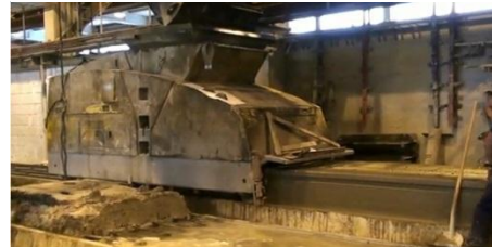
Picture 4 Steeping machine making hollow core elements on top of tension wires
