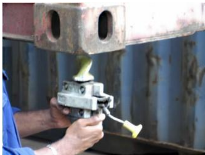
Figure 5.16: A stevedore is installing an automated twist lock (Spreaders 2008)
