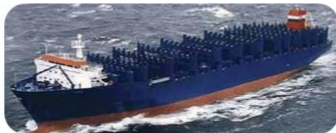
Figure 5.18: Container ship with no hatch covers
