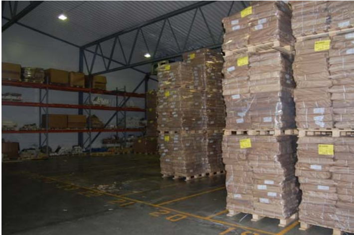
Figure 2-4 Tracks are identifiable areas for bulk storage inside a warehouse, see floor markings. Photo: O. Bø
