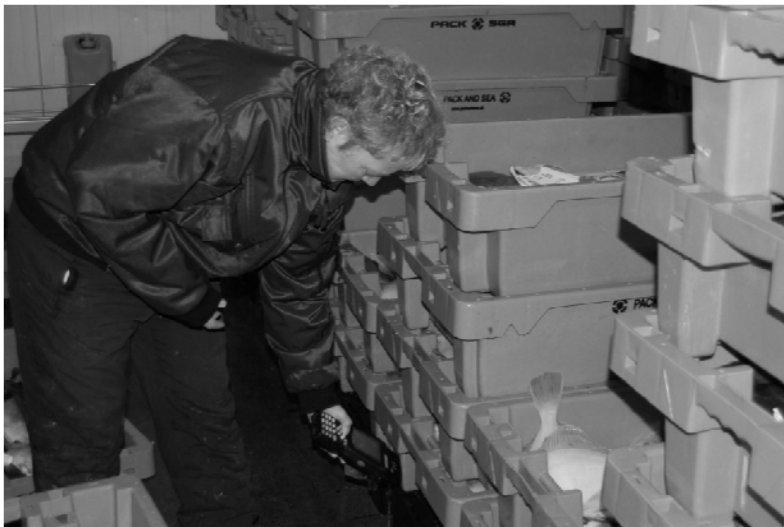
Figure 8-3 Using a handheld RFID reader to assign a fish box to a new owner. Low selectivity means that close range reading is necessary to select the right box (Case 2 fish auction). Photo: O. Bø
