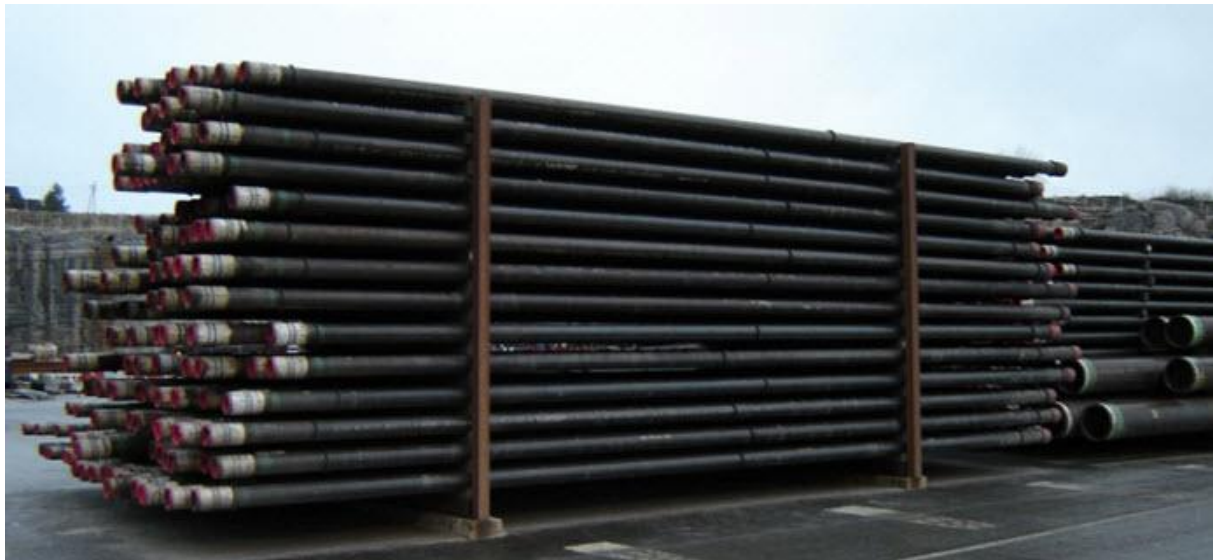
Figure 42 Casing pipe long term storage stack
