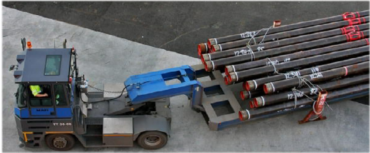
Figure 20 MAFI truck carrying pipe rams in lifting straps (source: Vestbase AS)
