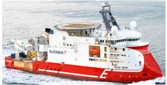
Figure 8 - Seven Viking: An inspection, maintenance and Repair vessel (IMR) used for subsea operations built by Ulstein for Eidesvik Seven AS (Ulstein.no 2014c)
