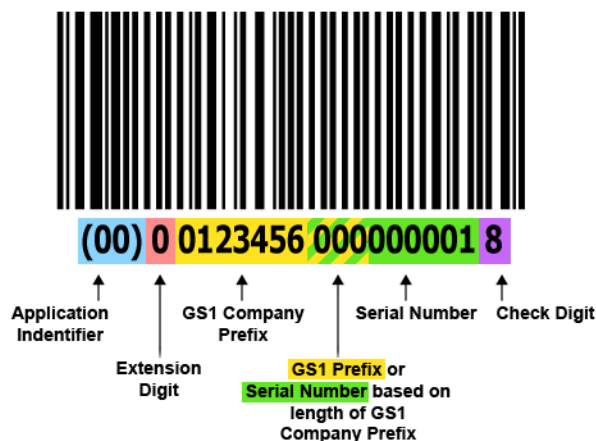
Figure 8 Example of a SSCC barcode and explanation
