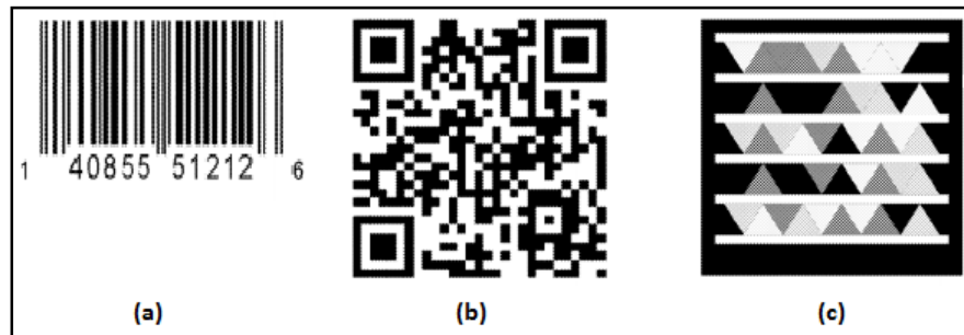
Figure 4. Examples of first (a), second (b) and third (c) generation barcodes (Source: adapted by author from Roman et al, 2013)
