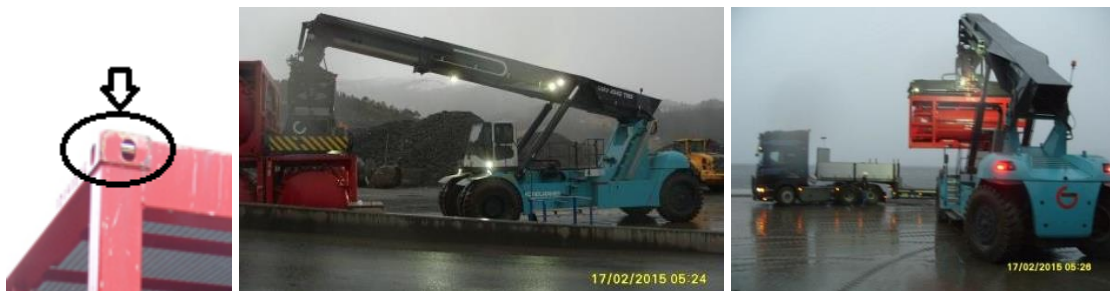
Picture 21: Handling of empty CTT by reachstacker at Husøya (Photo: Alexandra Boyarinova).
