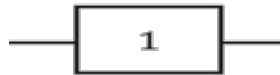
Figure 3. One device/component represented with reliability block diagram (RBD). Main principles of RBD and examples of the diagrams can be found in Goble (1998), Lewis (1996), IEC 61508 (1998-2005) and other resources.
