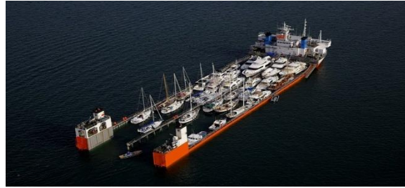
Picture 2.1: Float-on-Float-off ship (plusgoogle.com 2016)
