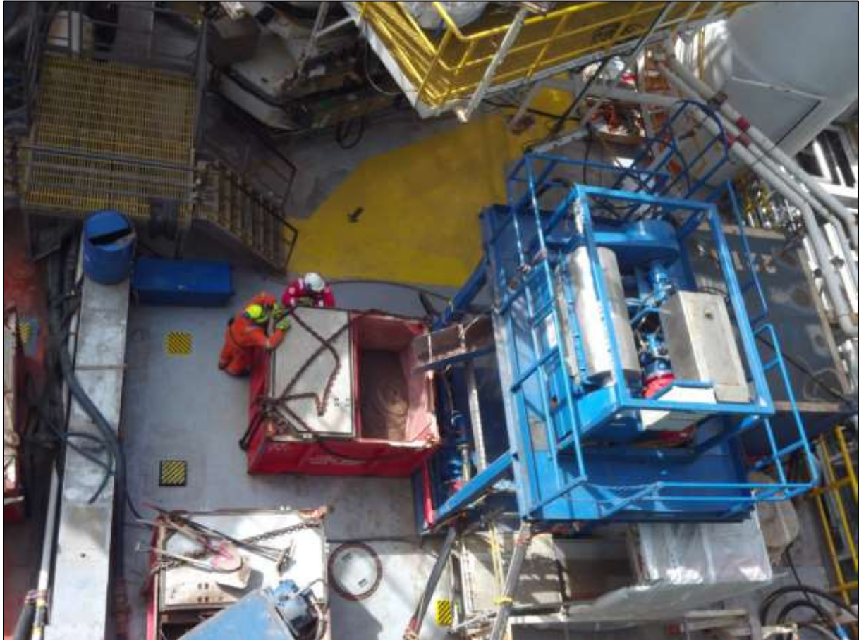
Figure 5-7 The centrifuge device in the Edvard Grieg field. Source: Lundin Norway AS
