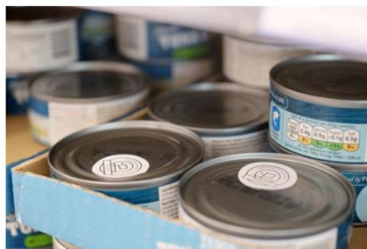
Figure 18: NFC Enabled smart stickers carry the Provenance mark along with item or Batch ID
