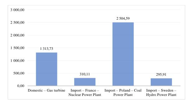
Figure 5-5 Annual CO<sub>2</sub> emission for Snøhvit – Europipe II pipeline chain, 10<sup>3</sup> ton/year
