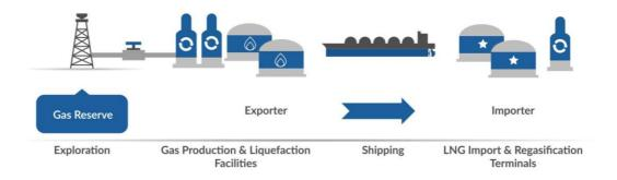
Figure 2-3: The life cycle of LNG. (Source: IGUb)
