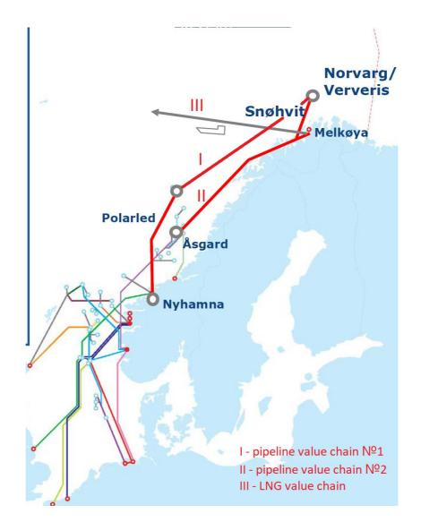
Figure 4-4 Potential gas transport solutions for the Barents Sea (Source: adapted from Lohne, 2013)
