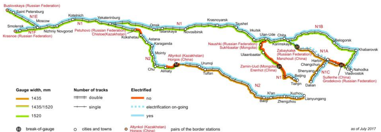
Figure 11: Railway infrastructure along the Eurasian Northern Corridor. Figure obtained from UNESCAP (2017).
