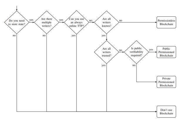
Fig. 1.: A flow chart to determine whether a blockchain is the appropriate technical solution to solve a problem (K. Wüst and A. Gervais)
