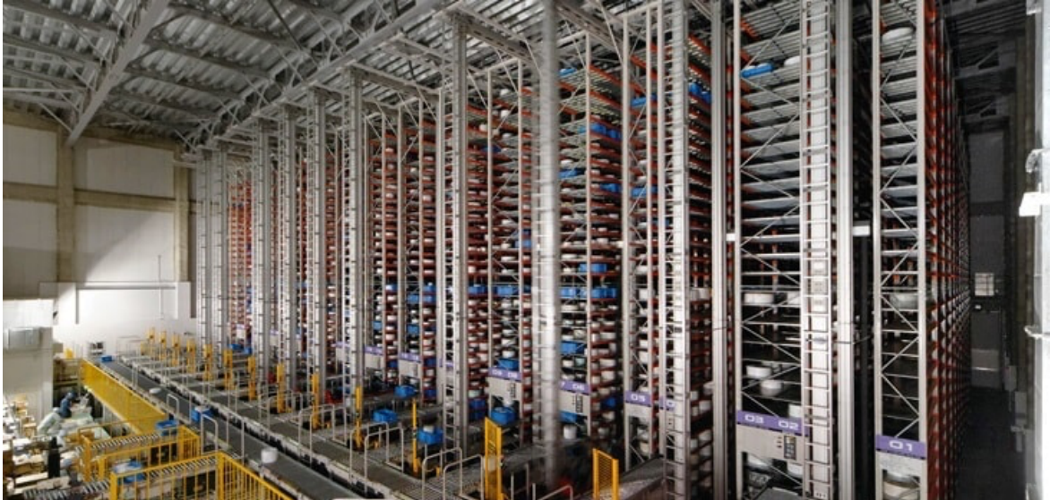
Figure 5 Example of AS/RS (Solutions 2021)
