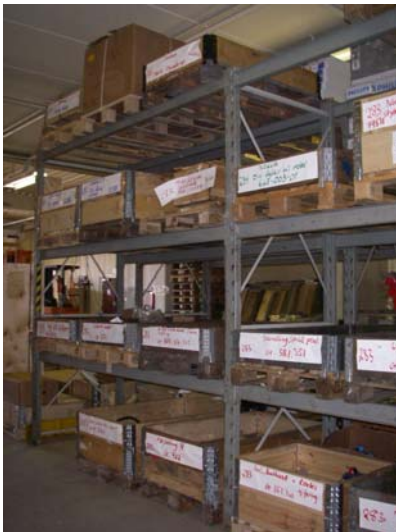
Pictures: Single-deep pallet racks in central warehouse
