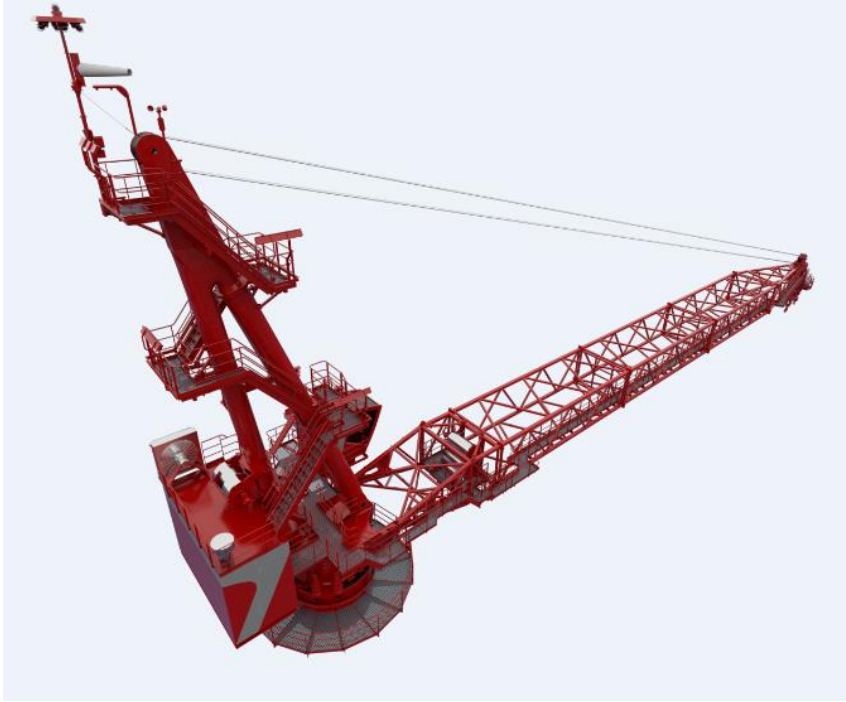
Figure 28 Picture of Lattice Boom Crane Z1318 Modularization project (National Oilwell Varco Norway AS 2014a)
