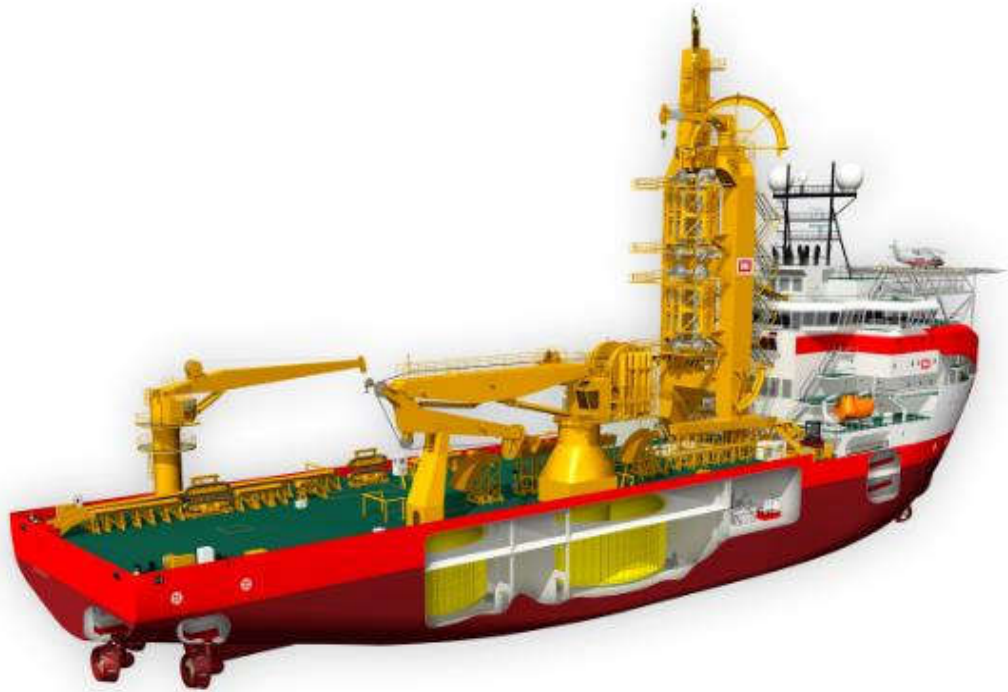
Figure 2.2 Pipe lay support vessel
