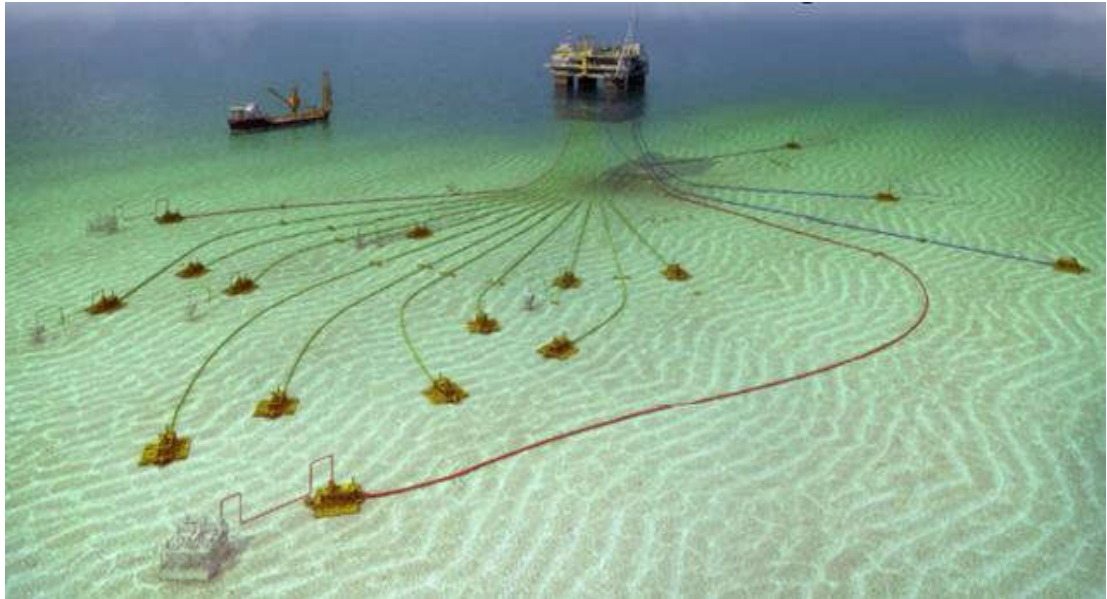
Figure 2.1 Pipelines connecting subsea wells and platforms
