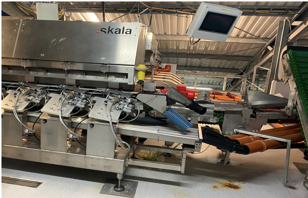
Figure 5.1. 2: Salmon vaccination machine (Source made by the Author of the master's thesis during her visit to the fish farm at Smøla).
