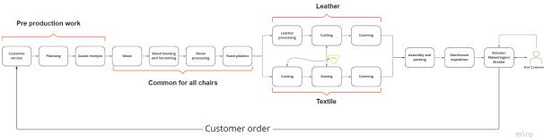
Figure 21 Process map of Ekornes production of Stressless dining chairs.
