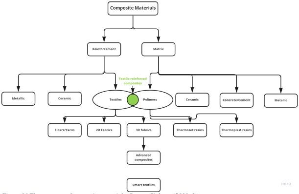
Figure 16 The structure of composite materials: Source Ciobanu (2011, 1)
