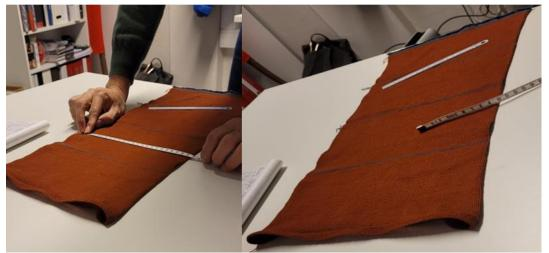
Figure 27 The technician measuring loop count in a test garment. The garment is seperated into different tightness in the different areas.
