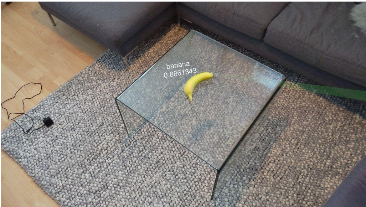
Figure 4.3: Example object label gets placed on the floor instead of the glass table, the numbers are the probability score of the class.
