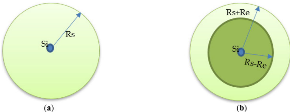
Figure 9. Sensing models. (a) Binary model. (b) Probabilistic model.
